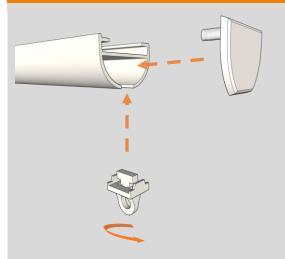
Attach the second stopper and end cover to the other end of the rail.
