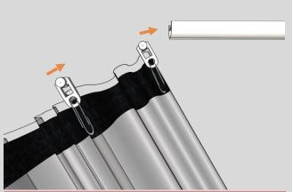
Guide the rollers into the rail one after the other, holding the curtain with the other hand to reduce the tensile load on the first rollers.
