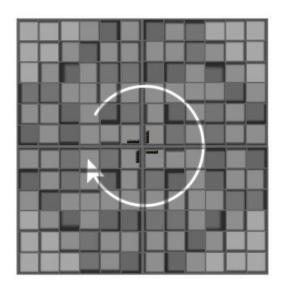
**Four diffusors** can be easily combined to form one **large diffusor**. To do this, the highest tiles must be rotated towards the corners.
