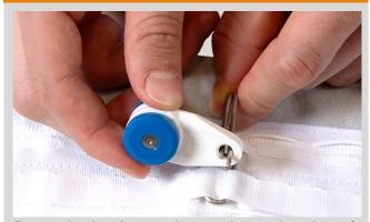
Press the hook together at the end and put it in the roller.
