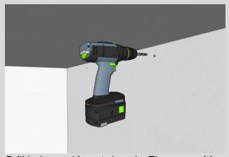
Drill holes and insert dowels. Then reposition the rail so that the dowels are visible in the holes provided in the ceiling mount.
