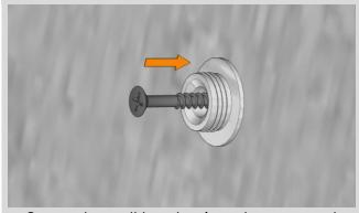
Screw the wall bracket into the prepared dowel.
