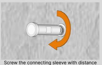
Screw the connecting sleeve with distance piece and magnet onto the wall plate.
