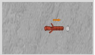
Now drill holes and insert suitable dowels.
