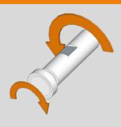
Screw the magnet into the distance piece.
