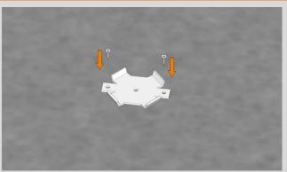
Now screw the metal plate of the mounting system onto the marked drill points on the wall sail.
