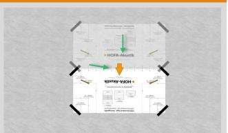
**Only for Wall Sail** 120: For the drill points on the opposite half, turn the template, attach it to the new position and mark the last drill points.
