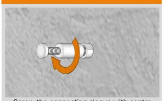
Screw the connecting sleeve with centre connection and magnet onto the wall plate. Then adjust the desired wall clearance by turning the threaded elements.
