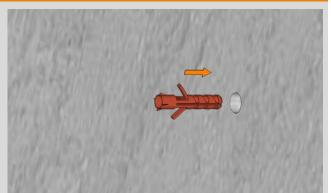
Now drill holes and insert suitable dowels.
